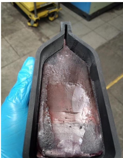
Fig.2. The large-sized single crystal \text{La}_{1-x-y}\text{Ba}_x\text{Pb}_y\text{F}_{2,94} ( x = 0,44 ; y = 0,06 ) synthesized by the HDS method in the graphite crucible with a \text{PbF}_2 content of about 6% (mol).
